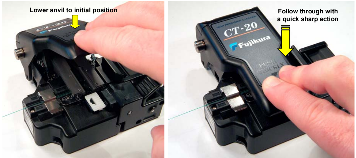
Figures 4.18 & 4.19 – Cleaving action
